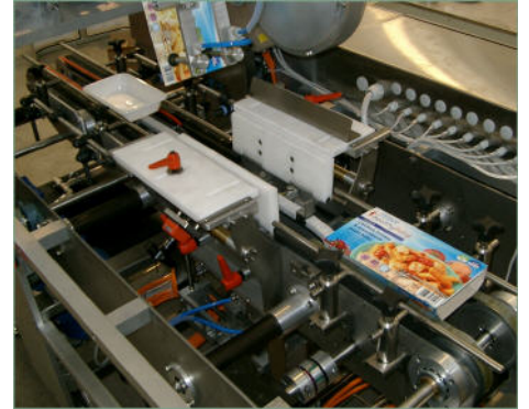
Tray & sleeve exiting the loading area
